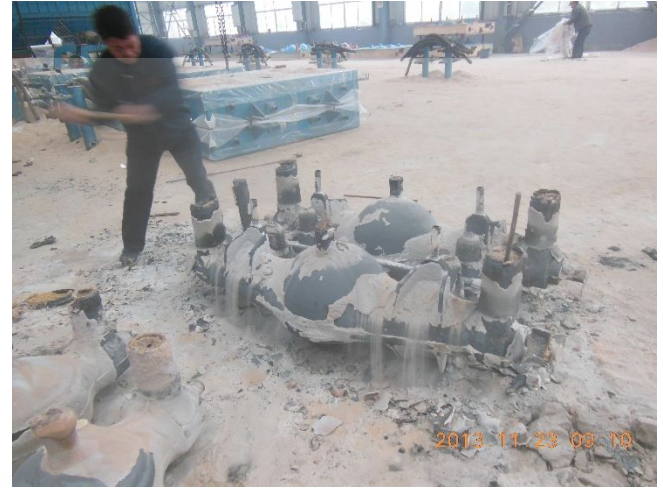
casting after shaking out
