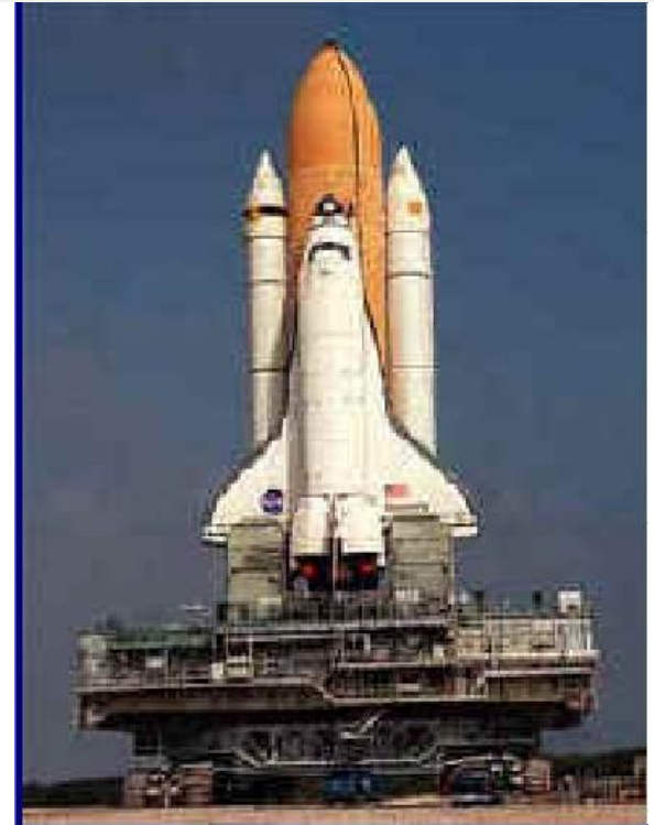
NASA Crawler Transporter with Space Shuttle (NASA Photo)
