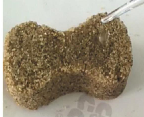
General modified Sodium Silicate sand
